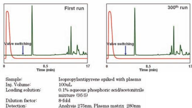
**Fig. 2 Evaluation of the Durability of the Shim-pack MAYI-ODS**
