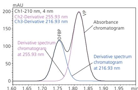
Fig. 5 Peak separation in the mixed sample (DFBP/VP=100/200)
