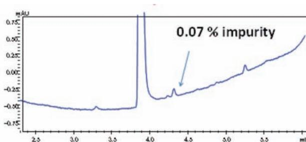
Fig. 10 Chromatogram for Indomethacin Using Normal LC Analysis
