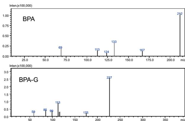
Fig. 2. Negative ion electrospray product ion tandem mass spectra of the deprotonated molecules of BPA ( $m/z$  227) and BPA-G ( $m/z$  403). The two most abundant product ions of each were selected for use during SRM.
