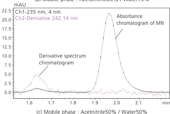
Fig. 3 Absorbance chromatogram and derivative spectrum chromatogram
