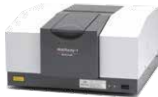
Shimadzu IRAffinity-1 FTIR Sistemi
