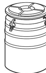
Flat-bottom, linear low-density polyethylene (LLDPE) drum with lid
