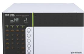
The RID-20A incorporates an auto purge function for the reference cell and a validation support function, consistent with the stability and expandability of Prominence HPLC series.
