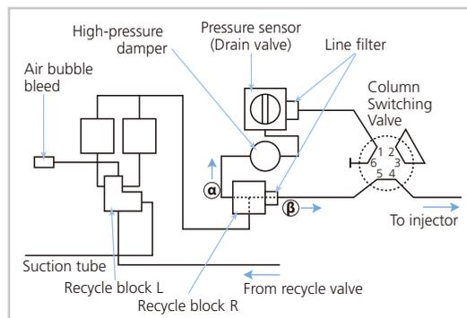
Flow Line Diagram of a Recycle Kit
