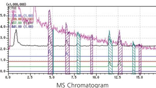
In preparation based on MS chromatograms, because the masses of the target compounds are specified, reliable fractionation is possible with simple fractionation conditions.
