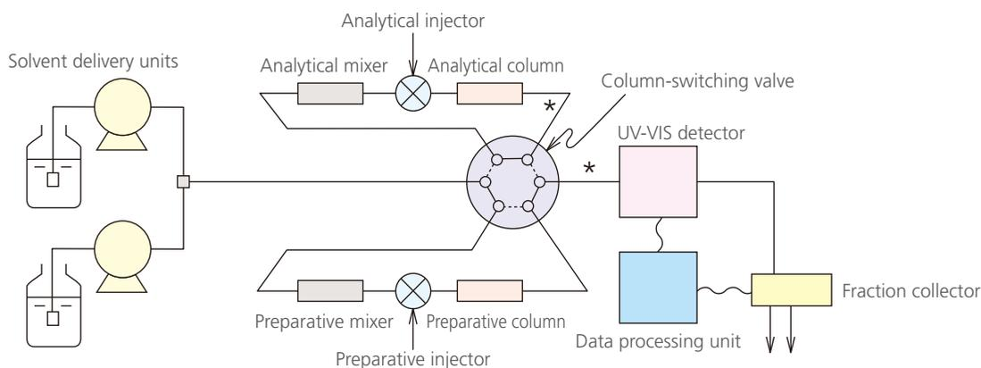
\* Analytical samples pass through piping created with 0.3 mm inner diameter tubes.
