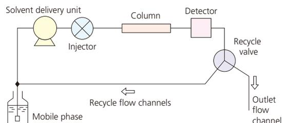
Flow Channels Used for Closed Loop Recycling
