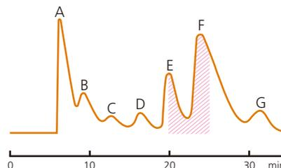
When the fractionation function of the FRC-10A is used, the target components can be reliably fractionated, even if the retention time varies.
