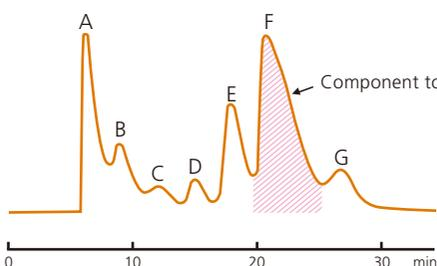
With time-based fractionation, the incorrect part is fractionated.
