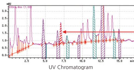
Fractionation performed using UV chromatograms depends on retention times and peak integration. For this reason, not only are the fractionation conditions complex, but the peaks for components other than the target compounds are fractionated, and high-efficiency preparation may not be possible.
