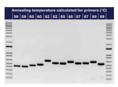
Figure 2. PCR amplification with high specificity and yield following a universal annealing temperature at 60°C. Primer sets with varying annealing temperatures were used to amplify 12 targets from human genomic DNA (gDNA) with a 60°C annealing temperature.
