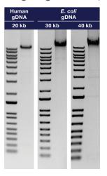
Figure 5. Amplification of long fragments. A 20 kb target from human gDNA and 30–40 kb targets from *E. coli* gDNA were successfully amplified by Platinum SuperFi II DNA Polymerase.
