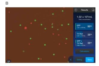
Figure 3. Rodent PBMCs accurately counted with machine-learning algorithm. The Countess 3 FL Automated Cell Counter was used to count small rodent PBMCs. Counts were performed with (A) brightfield lighting and (B) fluorescence lighting.
