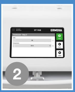
**Step 2:** Configure RPM and Temperature parameters of your dissolution run.
