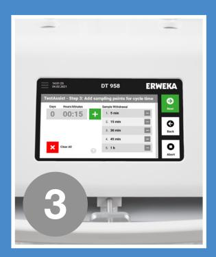
**Step 3:** Configure cycle times with a simple, yet effective input screen.
