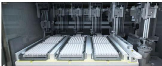
The Nexera MP system is able to access samples via the quickest path by moving the needle in both X and Y directions simultaneously. This achieves higher injection speeds than ever before, with shortest injection time being about 7 seconds.
