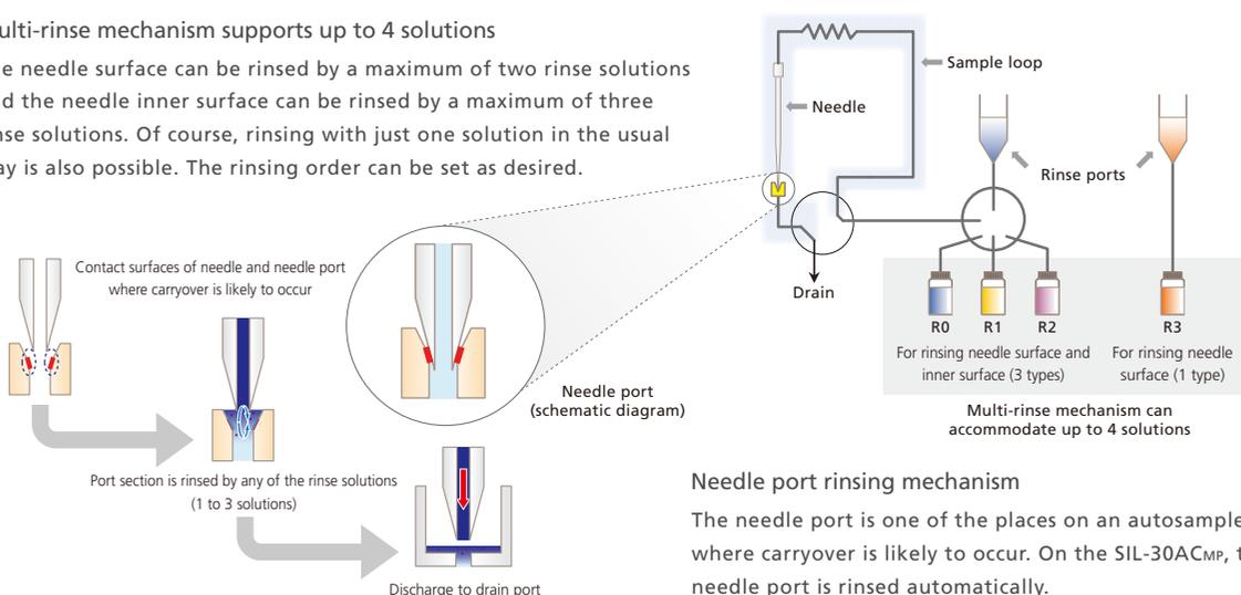
HPLC detectors, such as mass spectrometers, are becoming increasingly sensitive each year. Consequently, the carryover levels required for HPLC systems are becoming extremely strict. Nexera X2 series SIL-30AC and SIL-30ACMP autosamplers offer the ultimate in low-carryover performance, due to the thorough carryover-reducing mechanism.
