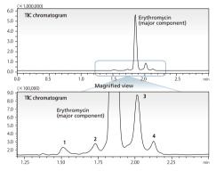
Using in-source CID allows the generation of fragment ions. This example shows the structure of impurities in erythromycin estimated from fragment ions generated by in-source CID. The multi-sequence mode permits several other methods within a single analysis, such as CID, positive/negative ion switching modes, and SCAN/SIM modes.
