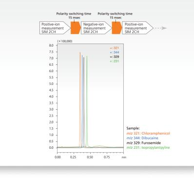
Accurate mass analysis of sharp chromatographic peaks obtained by UFLC requires ultra-fast MS detection capabilities.
