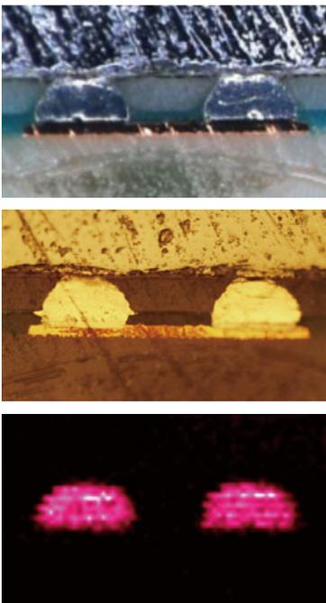
In the example shown on the left, imaging mass spectrometry technology is used to analyze the causes of soldering defects or contaminants on printed circuit boards.
