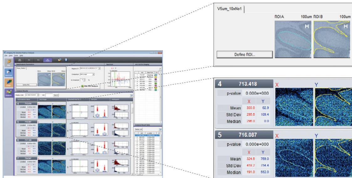
ROI analysis helps investigate and compare substances in two specified regions of interest (regions A and B, in the example above) to determine which substances are increased or decreased in each region. For example, if the amount of a given molecule increases in a cancerous region, then that is treated as a candidate cancer biomarker.
