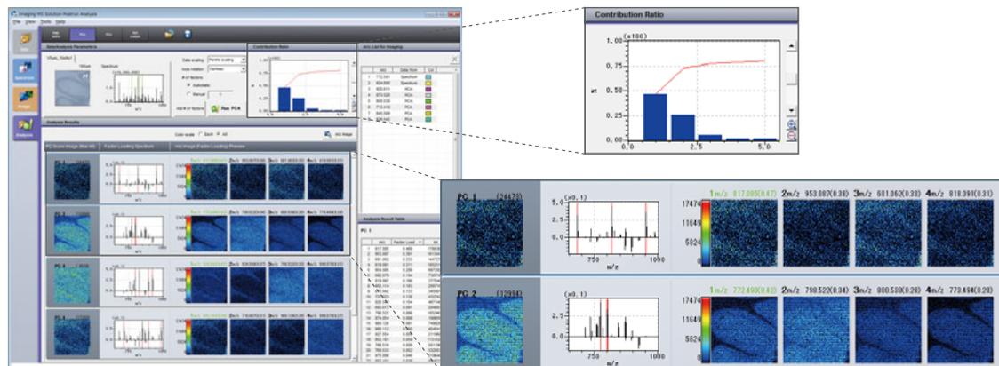
PCA organizes all detected peaks ( $m/z$  values) based on loading factor (weight coefficients assigned to individual peaks). When the peaks are arranged in an array, the MS images can form several patterns representing principal components. Therefore, PCA can be especially useful for finding ions that show specific localizations. This feature helps provide more multifaceted data analysis.
