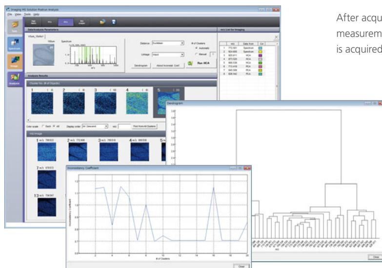
After acquiring an optical microscope image, measurement regions are specified and data is acquired by imaging mass spectrometry.
