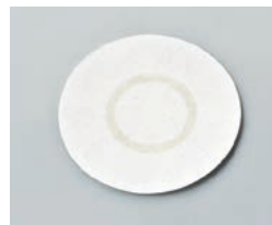
Perform measurements on sample dripped onto special filter paper and dried.
