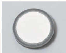
Press form the powder with a press machine (briquette press method).
