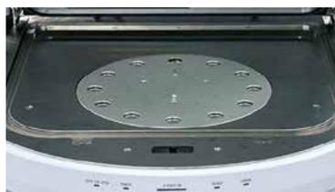
With the turret guide removed, samples varying in size can be added.
