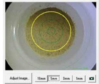
5 mm dia. Collimator Selected, Using Micro X-Cell
