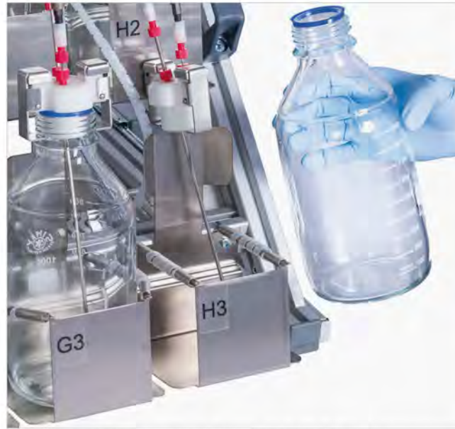
Easy filling of the sample rack with sample bottles
