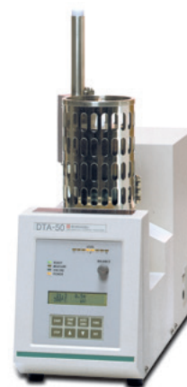
Measurement of the Moisture Content of PET Fiber (using a quartz crucible)
