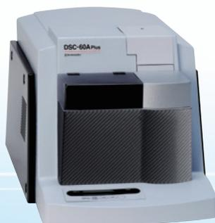
The built-in compact autosampler permits automated measurement, analysis, and report printout for up to 24 loaded samples. It improves the efficiency of screening during product development and the efficiency of quality control activities. The footprint is the same as the standard model.
