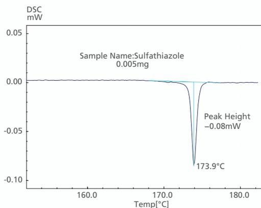
A stable baseline and S/N performance enable the detection of a minute calorimetric change during trace analysis.
