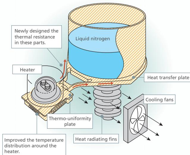
The new detector and new unique furnace construction achieves a noise level of less than 0.5μW, ensuring a stable baseline.
