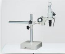
Optical Microscope Unit with CCD
