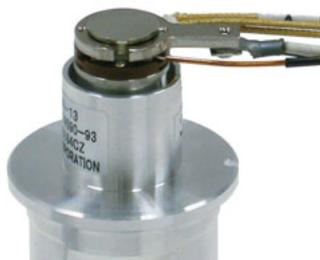
Heated Holder Installed in Scanner
