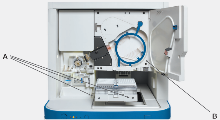
Figure 5. 3500 Series Genetic Analyzer. (A) Prepacked consumables, and (B) expanded capillary array.
